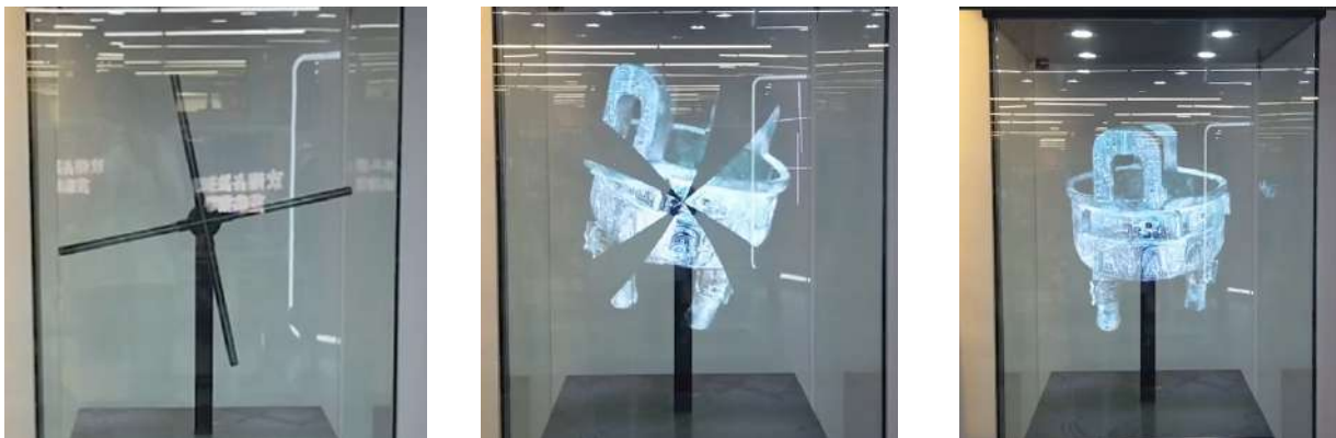
Gambar 1: Ilustrasi Prinsip Kerja Transmission Hologram ( https://medium.com/elektronhme )
