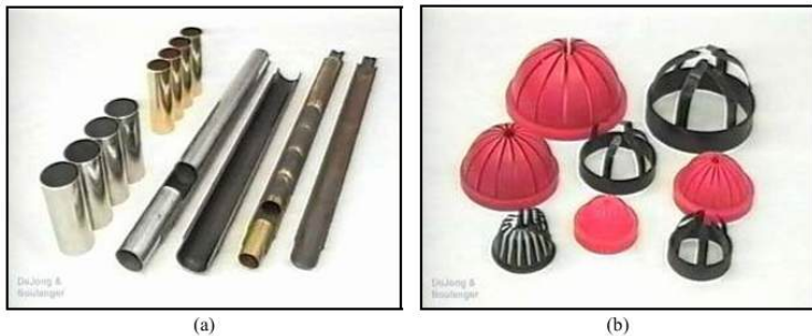
Gambar 3. 5 Split Barrel Sampler (a) Stainless steel and brass retainer rings (b) Sample catchers.
